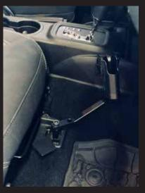
Slide the M12 X 90 mm cap screw through the top of the Mount Arm and then through the Spacer. Apply a small amount of threadlocker onto the screw threads and tighten the screw into the existing seat mounting hole. Prior to torquing the screw down, adjust the Holster Mount to the user desired location for optimal comfort and accessibility.
